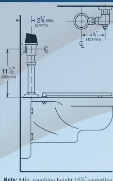
**Note:** Min. roughing height  $10\frac{1}{2}$  centerline of supply to top of fixture.
