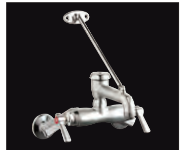
Service sink faucet with atmospheric vacuum breaker spout, model 445-VBRRCF
